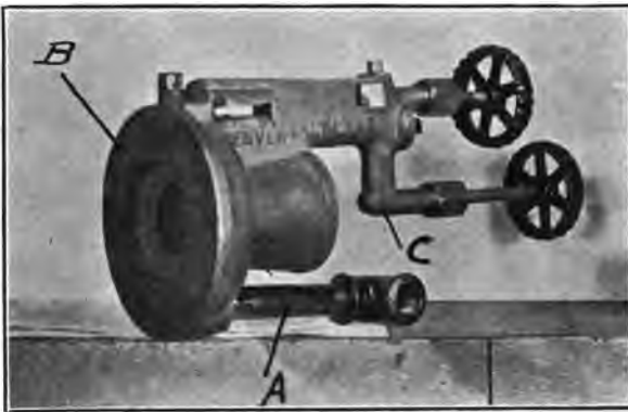
FIG. 18.—CASE-BURNER. A , Nipple containing gravel for straining gasolene; B , Generator; C , Valve.
